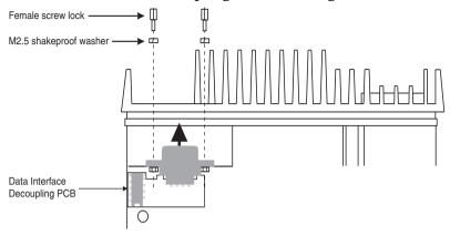
Fit the decoupling PCB to the T2000 chassis, from the inside rear of the radio, as shown.
